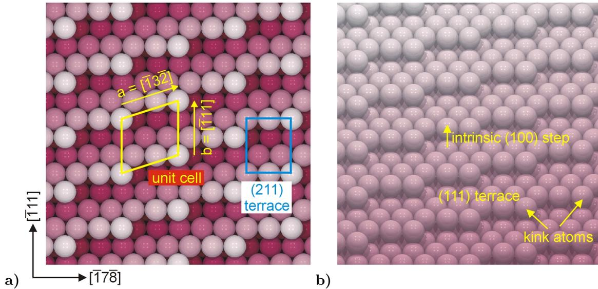
**Figure 3.3:** a) Hard-sphere model of the (532) surface
