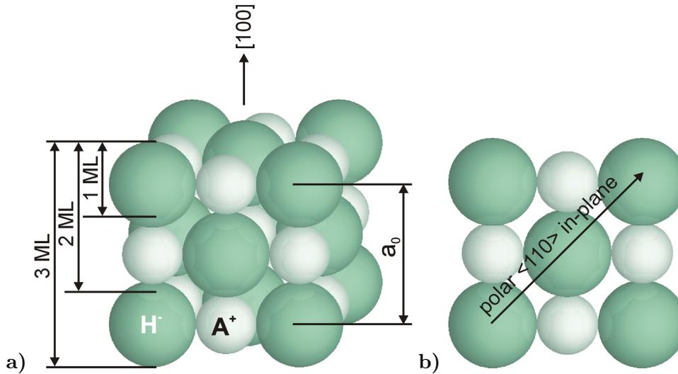
**Figure 3.5:** Hard-Sphere model for the rock salt structure of alkali-metal halides
