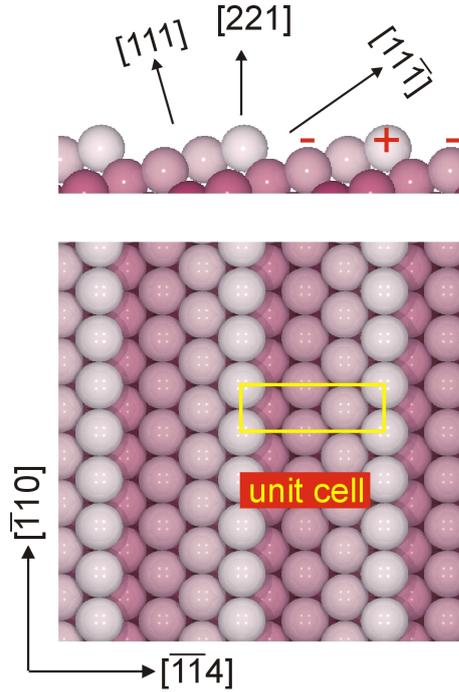
**Figure 3.2:** Hard-sphere model of the (221) surface
