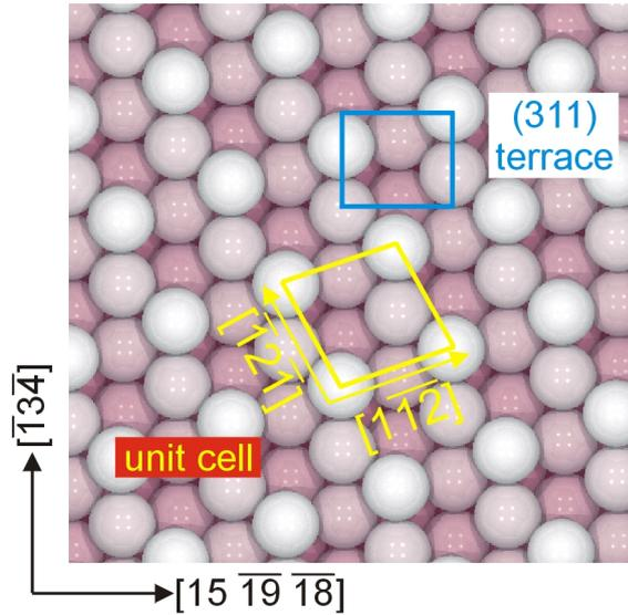
**Figure 3.4:** Hard-sphere model of the (531) surface
