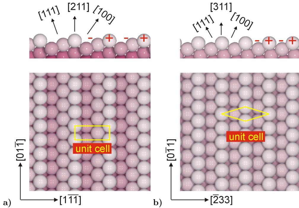
**Figure 3.1:** a) Hard-sphere model of the (211) surface
