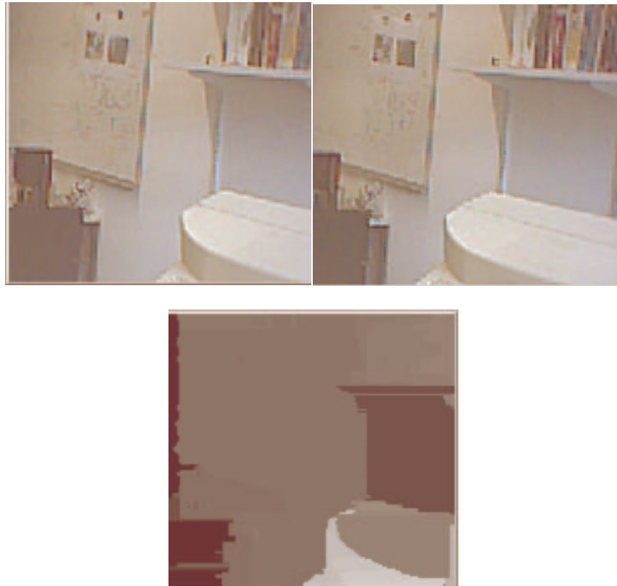
Figure 11.5: Results of the Cox algorithm. Right Image, left image and density stereo map.
