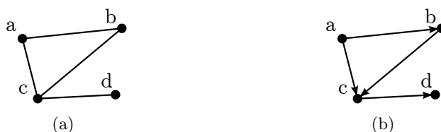
Figure 3.1 Graphs. (a) a simple graph G = (N, E) with N = \{a, b, c, d\} and E = \{\{a, b\}, \{c, a\}, \{c, b\}, \{c, d\}\} . (b) a directed graph D = (N, \vec{E}) with N = \{a, b, c, d\} and \vec{E} = \{(a, b), (a, c), (b, c), (c, d)\}
