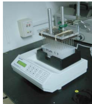
Figure 12: The Swizzler. An inverted 96-pin device assists resuspension of bacteria and mixing of solutions.
