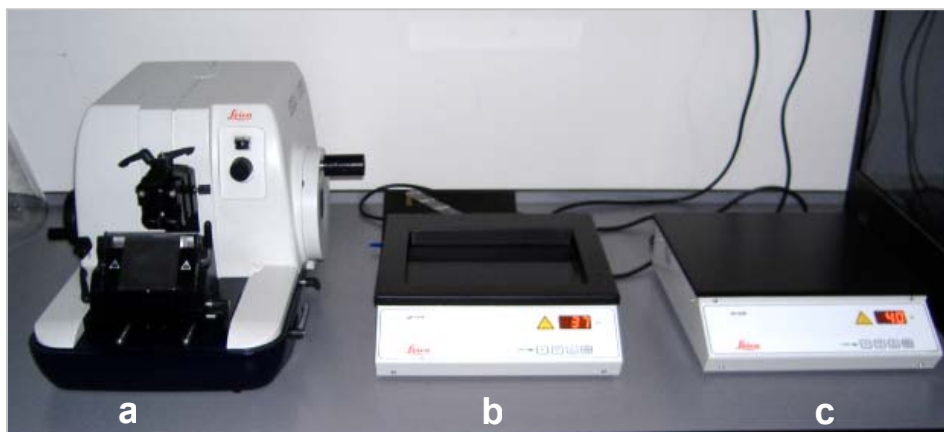
Figure 13. Equipment for cutting of paraffin embedded tissues: a) microtom, b) water bath, c) hot plate.
