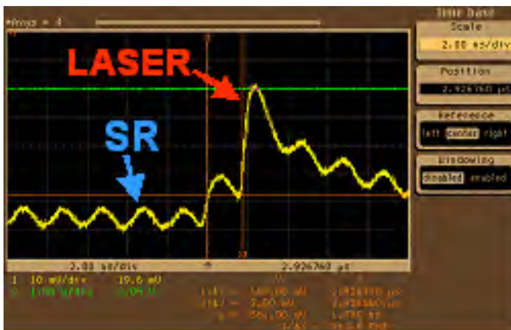
Figure 2.16: Signal of both laser and synchrotron pulses (in multibunch mode) on a fast photodiode monitored by a fast sampling oscilloscope (500 MHz bandwidth).
