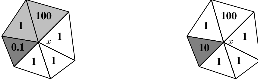
Figure 3.1: The distribution of coefficients k_T, T \subset \omega_x is quasi-monotone with respect to the node x on the left figure but not on the right one. The simplex T is colored dark and the set \tilde{\omega}_{T,x,qm} is colored with different levels of grey in the left picture
