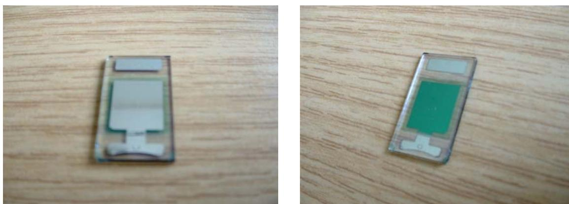
**Figure 71.** Photographs of the up-scaled solar cells, seen from the metal contact side (left) and through the glass (right). The green-blue coloring is the organic layer part of the cell
