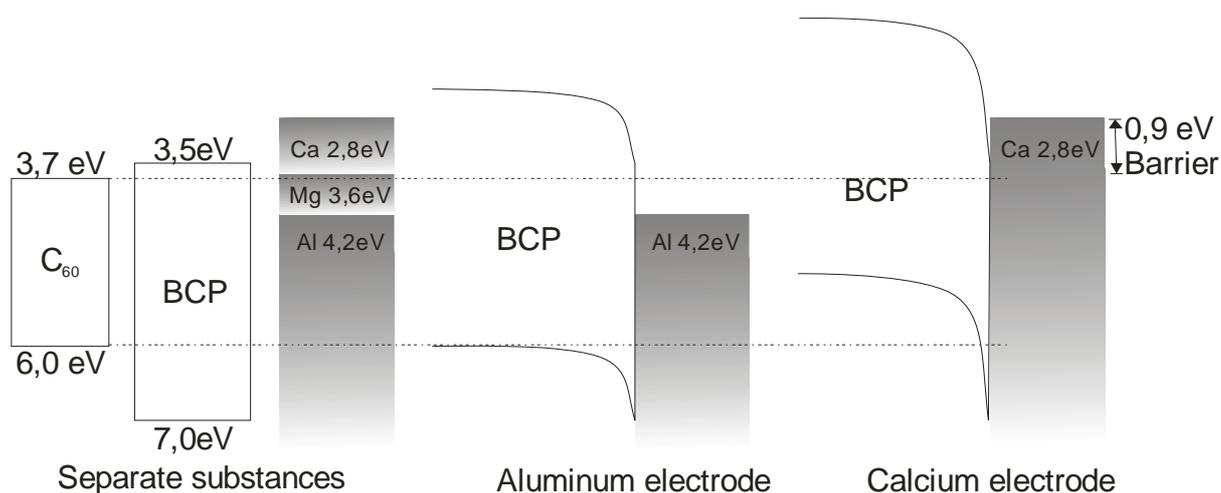
**Figure 64.** Band diagram section, visualizing the interface between back contact and C<sub>60</sub>, through the BCP buffer. Bending of the bands of BCP favors electron transport to Al, but creates an energetic barrier with Ca, as a back-contact (similar to Mg, not shown on the figure). Values for C<sub>60</sub> are obtained from [59] as measured by us, and differ from the ones shown on the general cell energy band diagram from literature, shown in 1.3
