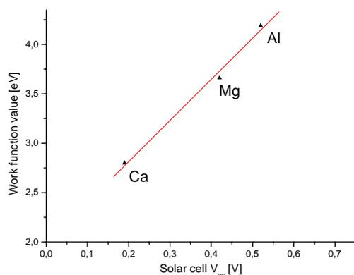
**Figure 63.** Plot of the work function of the metals Ca, Mg and Al against the corresponding solar cell  $V_{oc}$  achieved with these metals as back electrodes
