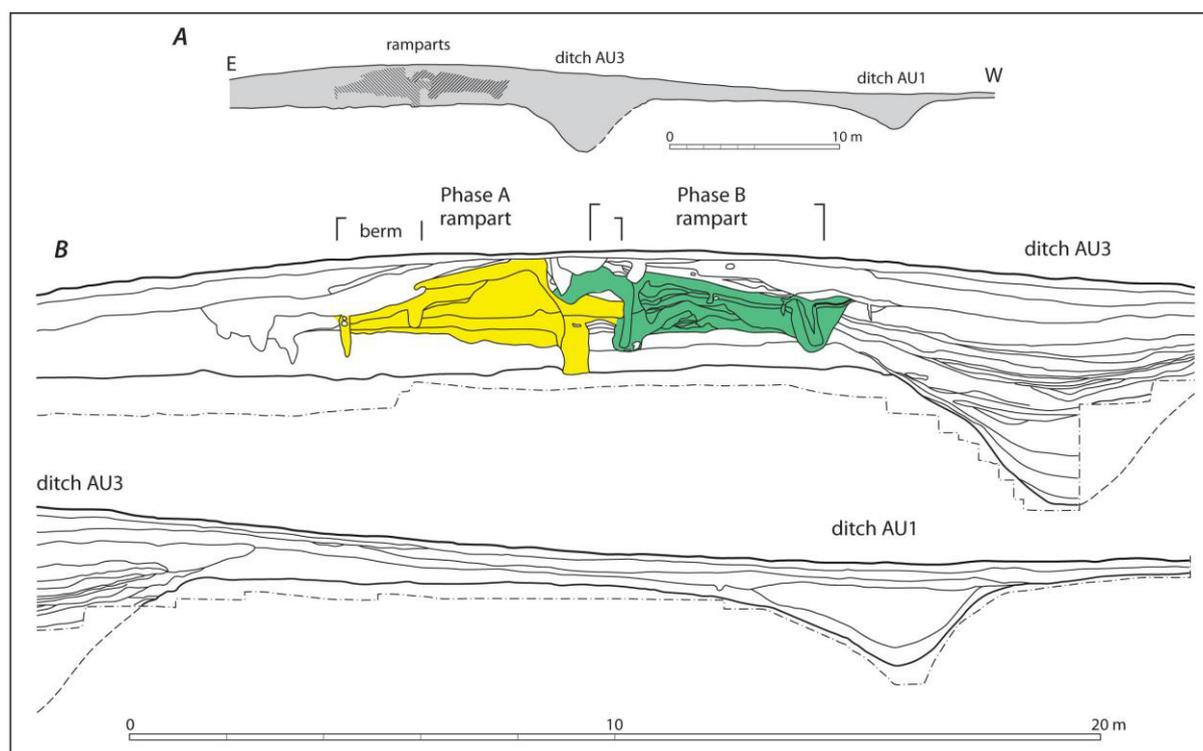
Fig. 17. A) Schematic representation of the excavation trench (trench 2 in Fig. 16) that cuts rampart I and the two defensive ditches in front. B) Detailed drawing of the trench indicating the two different construction phases (Phase A and B) of rampart I (Szentmiklosi et al., 2011).
