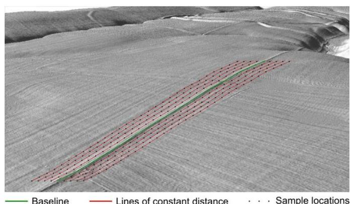
Fig. 27. Visualization of the applied method of generating topographic swath profiles. Lines of constant distance (red lines) are generated using the signed (oriented) distance to the defined baseline (green line); then samples from the underlying DEM are taken at defined intervals (black dots) along the lines of constant distance.
