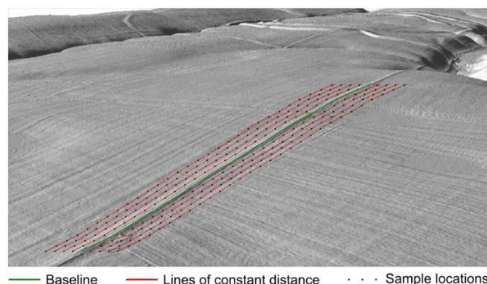
Fig. 24. Visualization of the applied method generating topographic swath profiles (Nykamp et al., 2017b).
