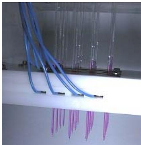
**Figure 4: Spotting head with 16 piezoelectric nozzles (courtesy of Dr. L. Nyarsik, MPIMG)**
