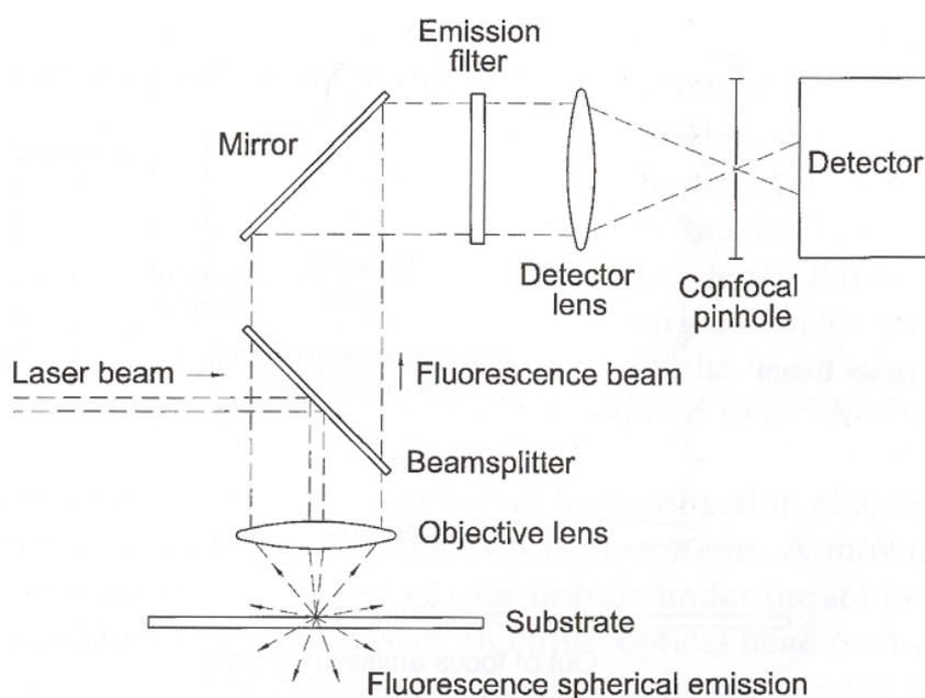
Figure 6: Principle of confocal scanner (35)
