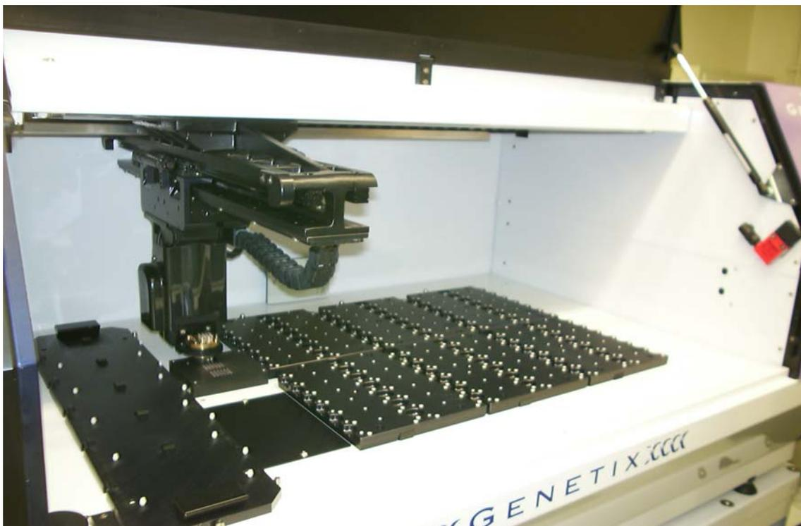
**Figure 2: Interior of spotting robot**
