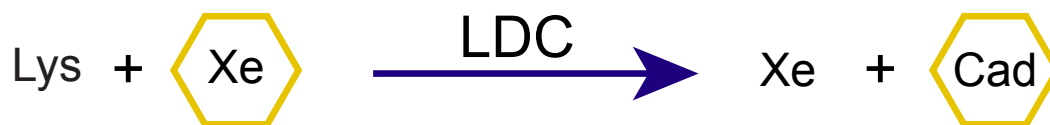
Figure 4.45 – Scheme of the LDC detection via Hyper-CEST. First Xe is encapsulated in CB (yellow hexagon) and Lys is in solution. The enzyme LDC produces Cad, which shows a higher binding affinity to CB than Xe.
