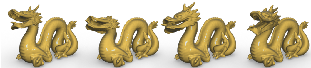
Figure 3.1: Reduced simulation of a geometrically nonlinear deformable object with 92k tetrahedra computed at over 120Hz after about four minutes of preprocessing (see Table 3.3).
