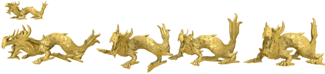
Figure 5.2: Linear vibration modes and modal derivatives of the Discrete Shells energy on the Chinese dragon model. Figure shows: the rest state (top left), two linear modes (left), and two modal derivatives (right).
