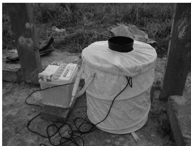
Fig. 3.5 Mechanical odour baited mosquito trap powered by a car battery – BG-Sentinel™ trap. Boadi Cattle Research Farm, Kumasi, Ghana 2005.
