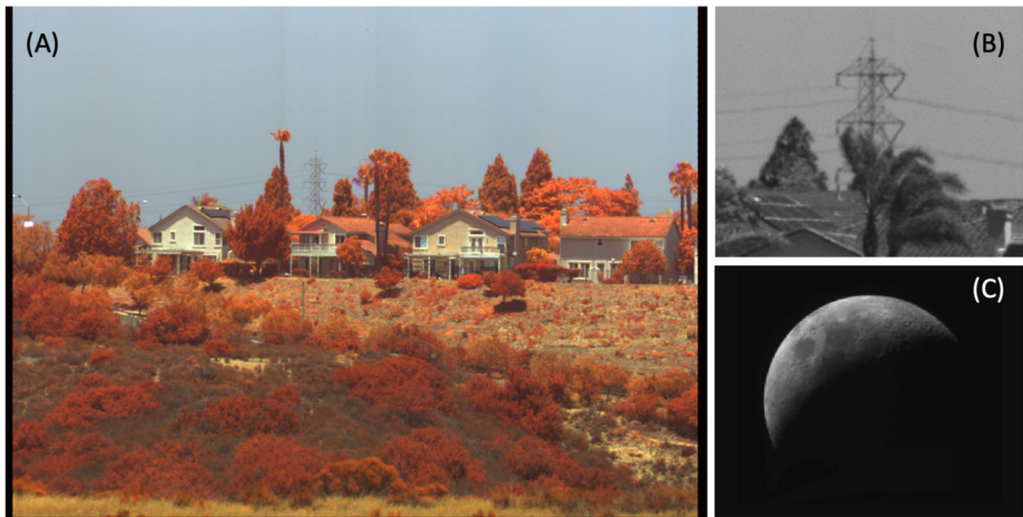
Fig. 6 Examples of “real world” imaging with Imager A in pre-flight testing at MSSS in San Diego. (A) Full frame ( 1648 \times 1200 pixels, including masked reference columns) color composite image of the view out a special cleanroom window of houses on a ridge \sim 1 km away. RGB = 722, 548, and 439 nm. (B) Enlarged 548 nm view of power lines \sim 2 km away and behind the houses, demonstrating good focus under typical terrestrial imaging conditions. (C) Subset of an Imager A night-time image of the Moon, acquired during relatively clear and dry conditions on Jan. 27, 2022 at 02:26 UTC. The Imager’s 50 \mu\text{rad} IFOV ( \sim 10 arcsec on the sky) corresponded to a scale of \sim 19 km/pixel on the Moon. Imager B performed similarly under terrestrial conditions
