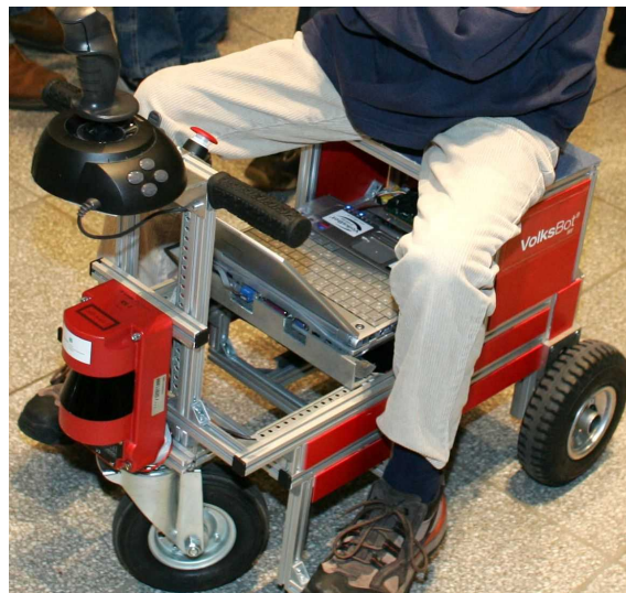
Figure 2.40: The PeopleMover, a prototype of an intelligent vehicle on VolksBot basis
