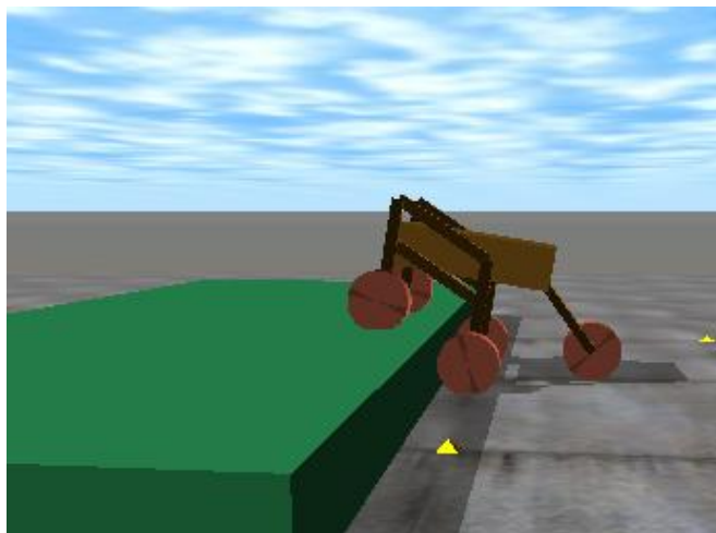
Figure 2.27: Simulation in ODE of the 5-wheeled XT
