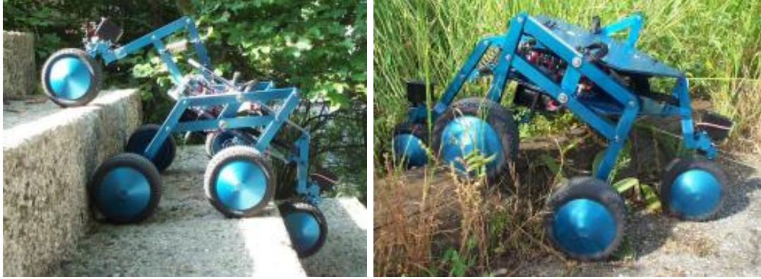
Figure 2.22: The Shrimp Rover (EPFL) adapting to rough terrain
