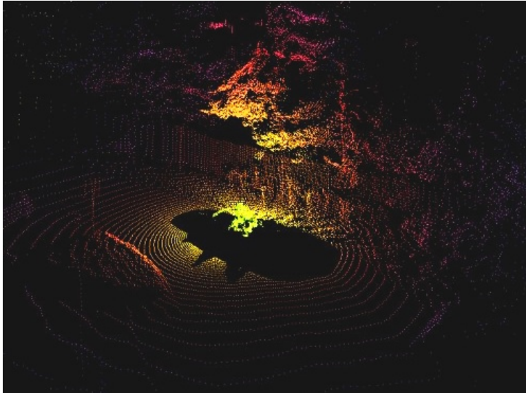
Figure 3.14: A resulting 3D scan from 3DLS-K with color coded distance values
