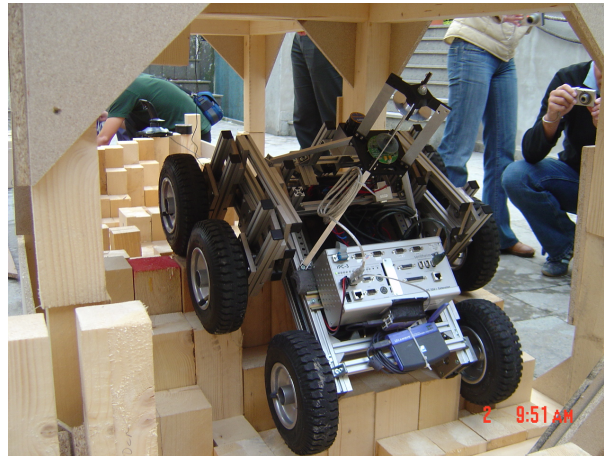
Figure 2.38: VolksBot XT traversing a random step field at the RoboCup Rescue Workshop 2005
