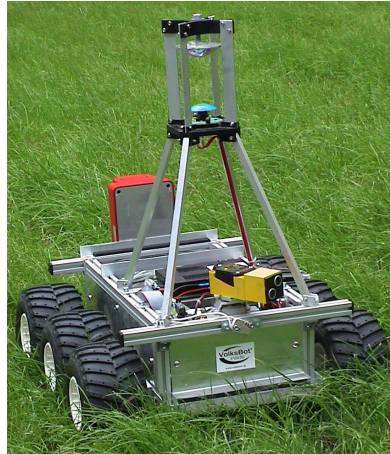
Figure 2.17: Pegasus - an outdoor rover equipped with VolksBot components
