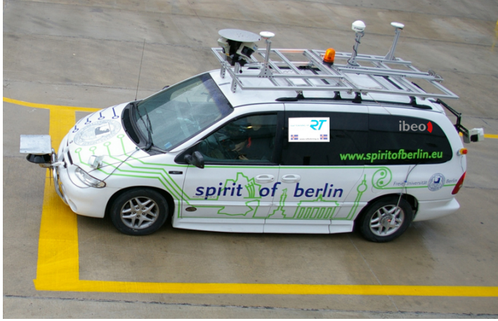
Figure 3.17: Spirit of Berlin with integrated Fraunhofer 3DLS-K LIDAR
