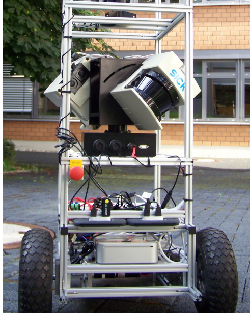
Figure 3.15: 3DLS-K as VolksBot sensor
