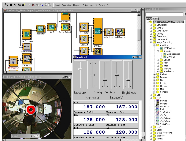
Figure 2.11: ICONNECT programming environment with graph, GUI and module library
