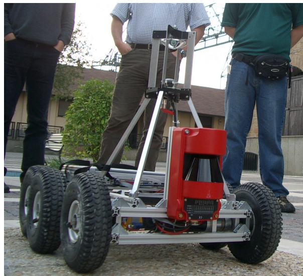
Figure 2.36: VolksBot RT6 used as a Rescue Platform at the RoboCup Rescue Workshop 2004 in Rome
