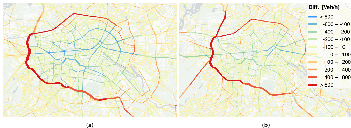
Figure 6. Differences in traffic load between scenario A and the base case for (a) 8–9 am and (b) 8–9 pm.
