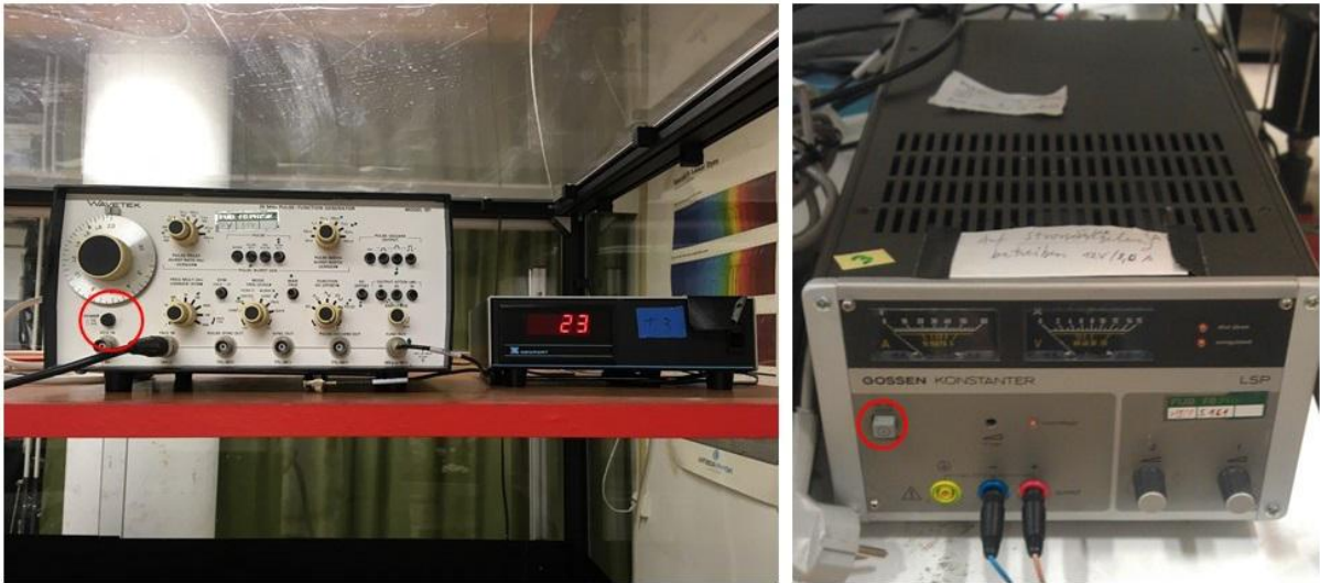
Figure: left: function generator and temperature measurement device. On the other side of the shelf, you find the voltage supply for the lamp (here shown on the right) and the oscilloscope.
