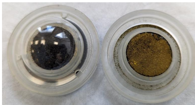
Figure 7.4. MAPbI 3 after 151 weeks stored in air.
