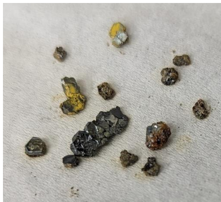
Figure 3.2. \text{MAPbI}_3 crystals obtained using the antisolvent method, the crystals were covered by \text{PbI}_2 .
