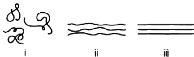
Figure 2-39 : Scheme of chains extension during the flow. i. Random coil, ii. Oriented chains by extension, iii. Pre-oriented chains have crystallized, adapted from Keller & Kolnaar., 2006.
