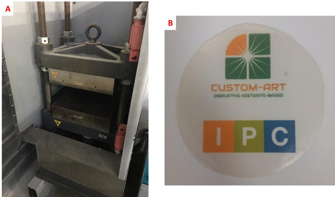
Figure 3-17 : a) Carver hydraulic press. b) Film made by compression molding with the C20A_5_5 blend.
