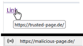
Figure 13. Example where both correct information and misleading information is shown at the same level of interaction for Link Mismatch in Mozilla Thunderbird.
