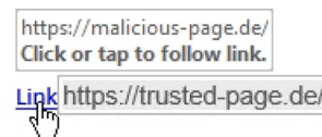
Figure 4. Example of “Fake Tooltip”. Displays both, fake (trusted-page.de) and original (malicious-page.de) tooltip as full-url at the same time.
