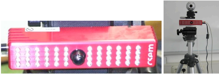
Figure 11.2: Left image: The SwissRanger time-of-flight 3D camera by CSEM. One can see the infrared light emitting diodes on both sides of the receiving lens. Right image: The camera stand that allows a 2D camera and the Swissranger to capture the same scene.
