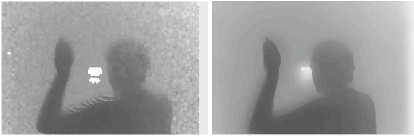
Figure 11.4: Left: Depth image obtained by the camera. Right: Depth image enhanced using the method proposed by [Diebel and Thrun, 2005]. The white spot in the center is an artifact produced by reflection.
