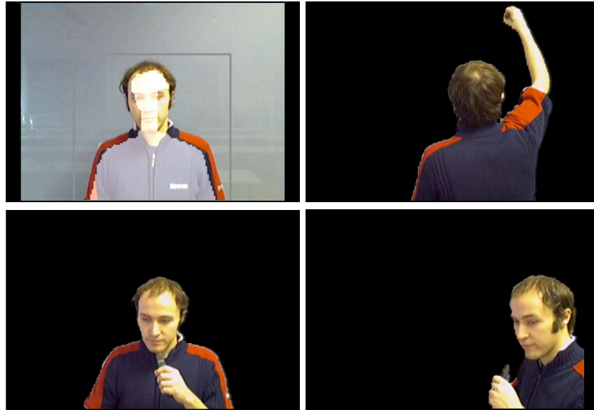
Figure 11.5: Top left: The depth data of the 3D camera is used to construct both a superset and a subset of the foreground. Other images: A few sample frames showing the segmentation result using the color segmentation approach described in the previous chapter. The instructor is robustly segmented while working with any content on the electronic chalkboard even if he or she is moving quickly. Results taken from [Santrac et al., 2006].
