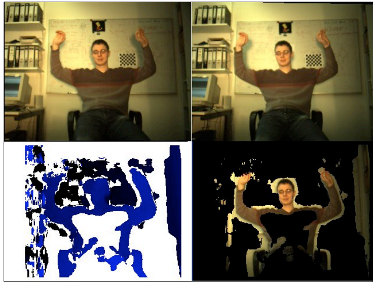
Figure 9.2: Using a stereo camera for segmentation. Top: Left and right views of the camera. Bottom left: Depth-range image, darker means farther away (white means unknown). Bottom right: Segmentation result by thresholding a certain depth, i. e., showing only pixels with depth coordinates in a certain interval. The experiment is described in the text.
