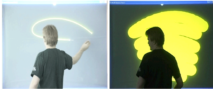
Figure 9.5: Worst case example of a change of lighting conditions during a lecture. Fortunately, such bad cases are very rare and can be reduced by using a proper configuration of the video camera.
