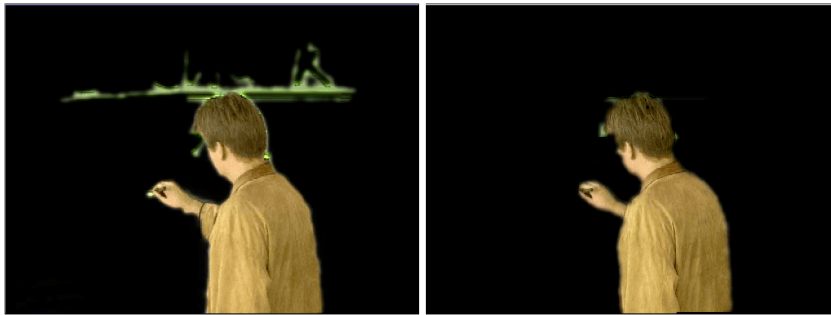
Figure 9.11: Board drawings that are connected to the instructor are often considered foreground by the classification. An additional board stroke suppression eliminates these artifacts. Left picture: The result of the color signature classification. Right picture: After applying a postprocessing step to eliminate board strokes.
