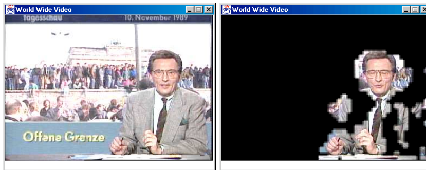
Figure 8.4: Visualization of the encoding of two consecutive frames from a TV broadcast (source: ARD, “Tagesschau”, November 10th, 1989): Blocks that have not changed significantly from the left frame to the right frame are colored black.
