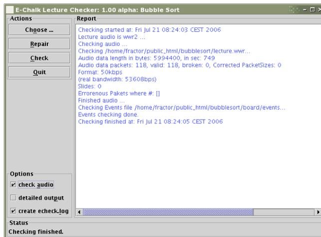
**Figure 6.1:** A screenshot of the E-Chalk lecture checker and repair tool. Audio recordings are scanned for broken packets and the file is repaired if possible.
