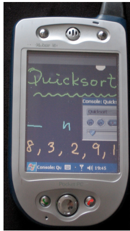
Figure 5.4: Java-based replay of an E-Chalk lecture on a mobile device running the PocketPC operating system (former Windows CE).
