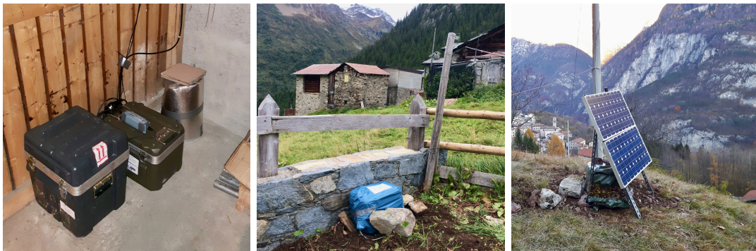
Figure 2.2. Examples of the deployment of different station types in the field. Online station (left), offline station (center), solar-powered station (right). All pictures were taken by me.
