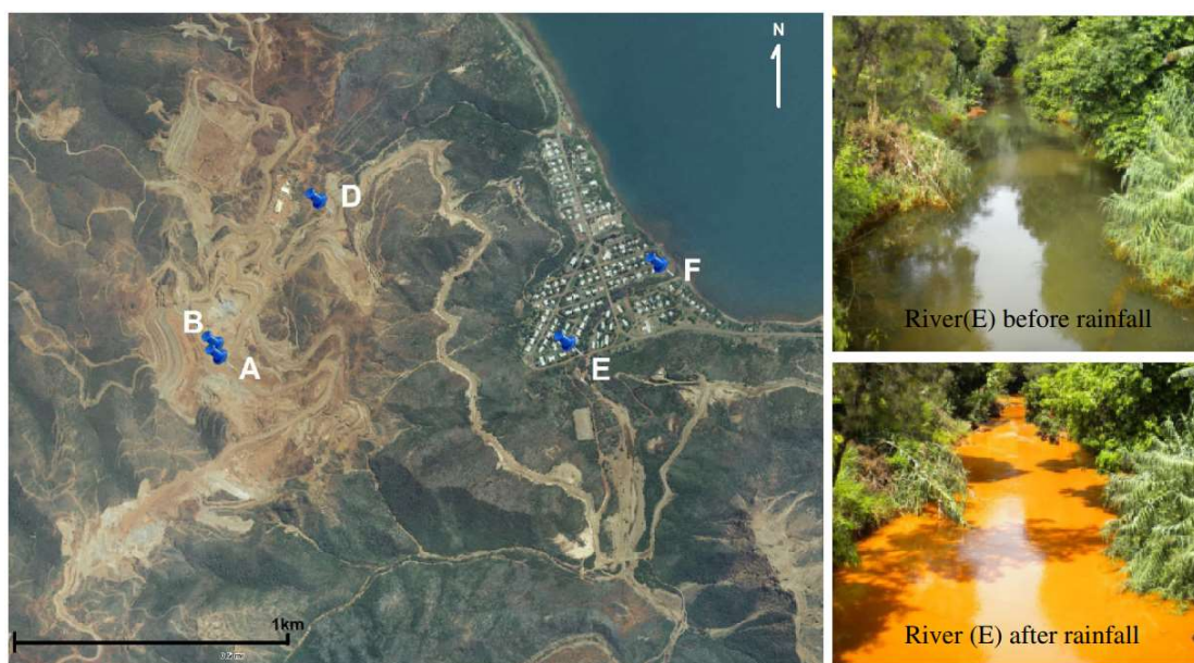
Figure 2.5. Mining area in Poro, New Caledonia showing the sites (A, B, D - mining catchment; river - E; river mouth - F) where high concentrations of Cr(VI) were measured, and images of the river before and after rainfall. Reproduced from Gunkel-Grillon et al. (2014) with permission from Springer Nature.
