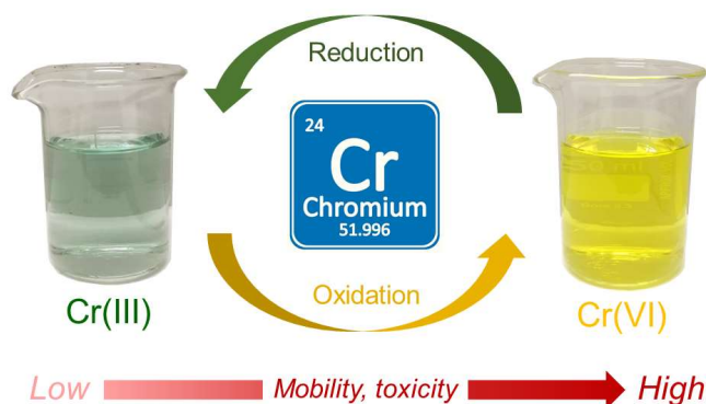
Figure 2.1. Diagram showing the contrasting properties of Cr(III) and Cr(VI). The green Cr(III) and yellow Cr(VI) solutions were prepared using \text{CrCl}_3 \cdot 6\text{H}_2\text{O} and \text{K}_2\text{CrO}_4 , respectively.
