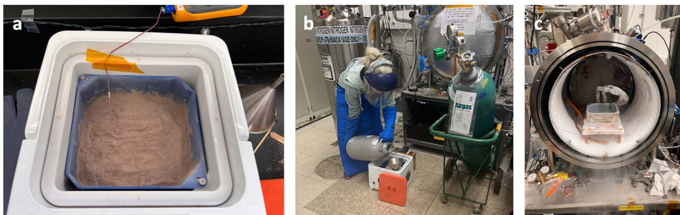
Figure 3. Methods used in each experimental run. Panel (a) shows the cryopod with basket filled with MMS dust and a thermocouple inserted to monitor cooling. Panel (b) shows the cryopod being filled with LN 2 , with DUSTIE in the background. Panel (c) shows the setup in the chamber just after an experiment has run and the door has opened. CO 2 frost coats all internal surfaces and is thicker on shroud and LN 2 hoses because these are at ~88 K owing to LN 2 flowing directly through them.
