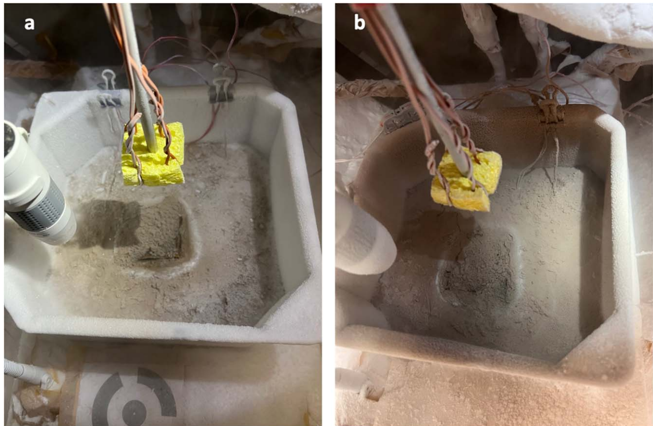
Figure 7. Bright halos observed in each experiment. An animation of their formation is available. This animation shows a bright “ring” gradually growing around the edges of the heater and increasing in brightness over time. The duration of the animation is 13 minutes and 45 s.
