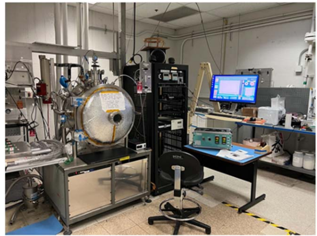
Figure 2. JPL’s DUSTIE thermal vacuum chamber.
