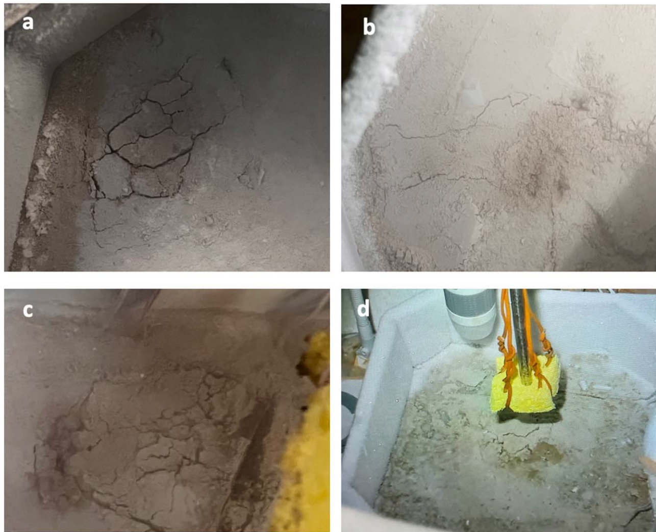
Figure 9. “Cracked” spider morphologies observed when heaters were stopped after plume activity began.
