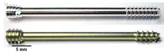
Fig. 1. 40 mm Mg-based orthopaedic compression screw MAGNEZIX® CS ø3.2 (top) and Ti market-equivalent (bottom).
