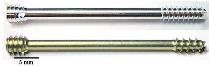
Fig. 1. 40 mm Mg-based orthopaedic compression screw MAGNEZIX® CS \phi 3.2 (top) and Ti equivalent (bottom), reproduced under the CC BY-NC-ND 4.0 License [9].
