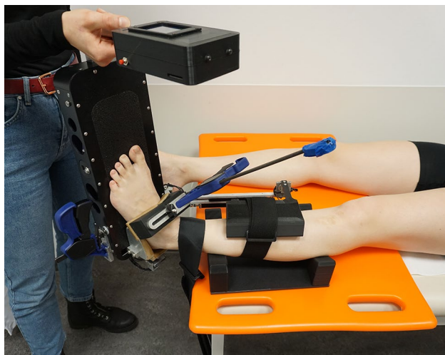
Fig. 3 Photo of the ankle arthrometer (Hollis Ankle Arthrometer™, Blue Bay Research, Inc., Florida, USA) and the experimental setup (a). The patient is lying on a stretcher, and the leg is positioned in the calf support on a hard pad and is fixed to the table proximal to the ankle joint. In this photo, an inversion test is being performed
