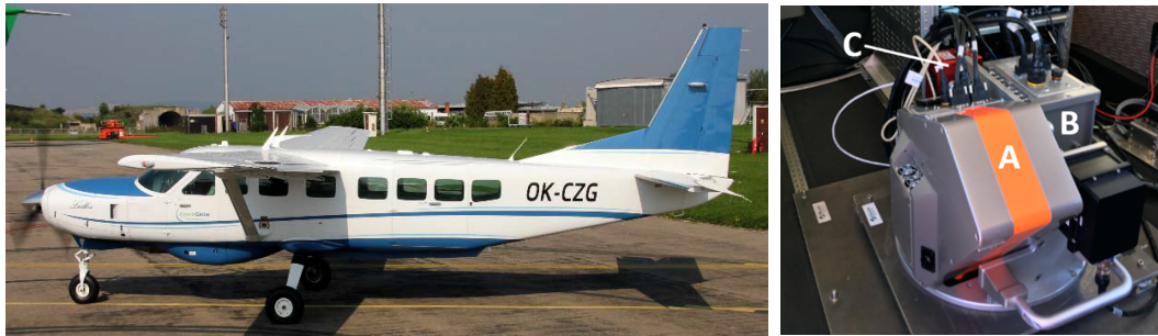
Figure 2.4 Left: Example aeroplane as measurement platform for HyPlant (Cessna Grand Caravan C208B Aircraft) taken from ESA [2020a]; right: image of HyPlant instrument with A pointing at the DUAL module, B at the FLUO module and C at the GPS/INS unit taken from Siegmann et al. [2019].
