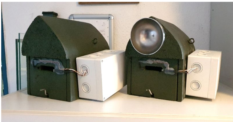
Figure 1. Gable boxes without and with an attached hollow hemisphere as an echo-reflective cue. The waterproof box located on the side houses the electrical components and power supply for the light beam system. Meanwhile, the diodes that measure interruptions, and thus bat activity, are affixed to both sides of the box entrance.
