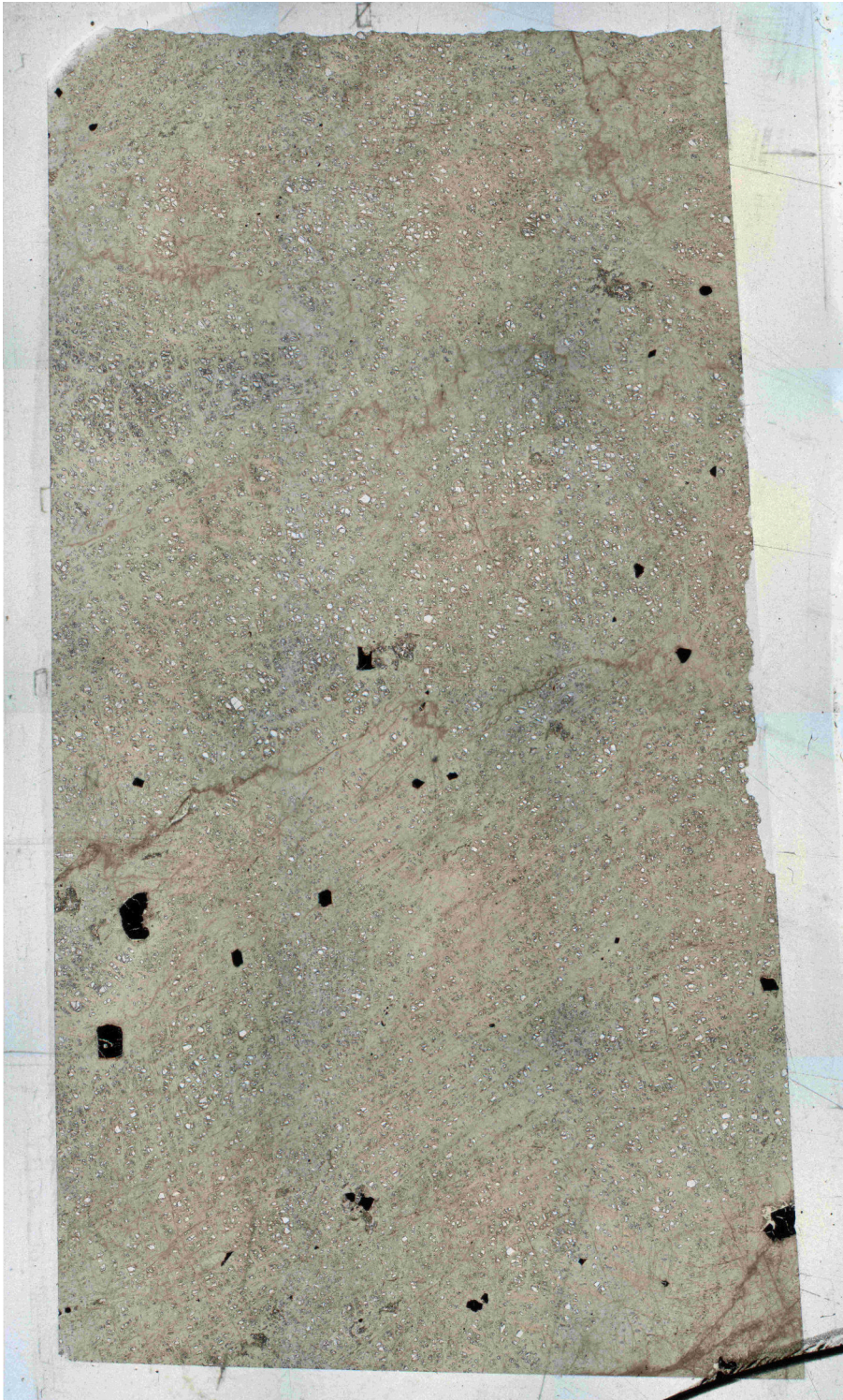
Figure A.5: Full thin section photography of sample ALB06-1 (serpentinized dunite).
