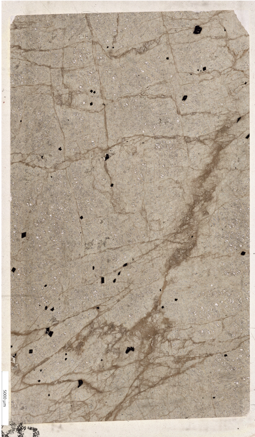
Figure A.6: Full thin section photography of sample ALB06-2 (serpentinized dunite).
