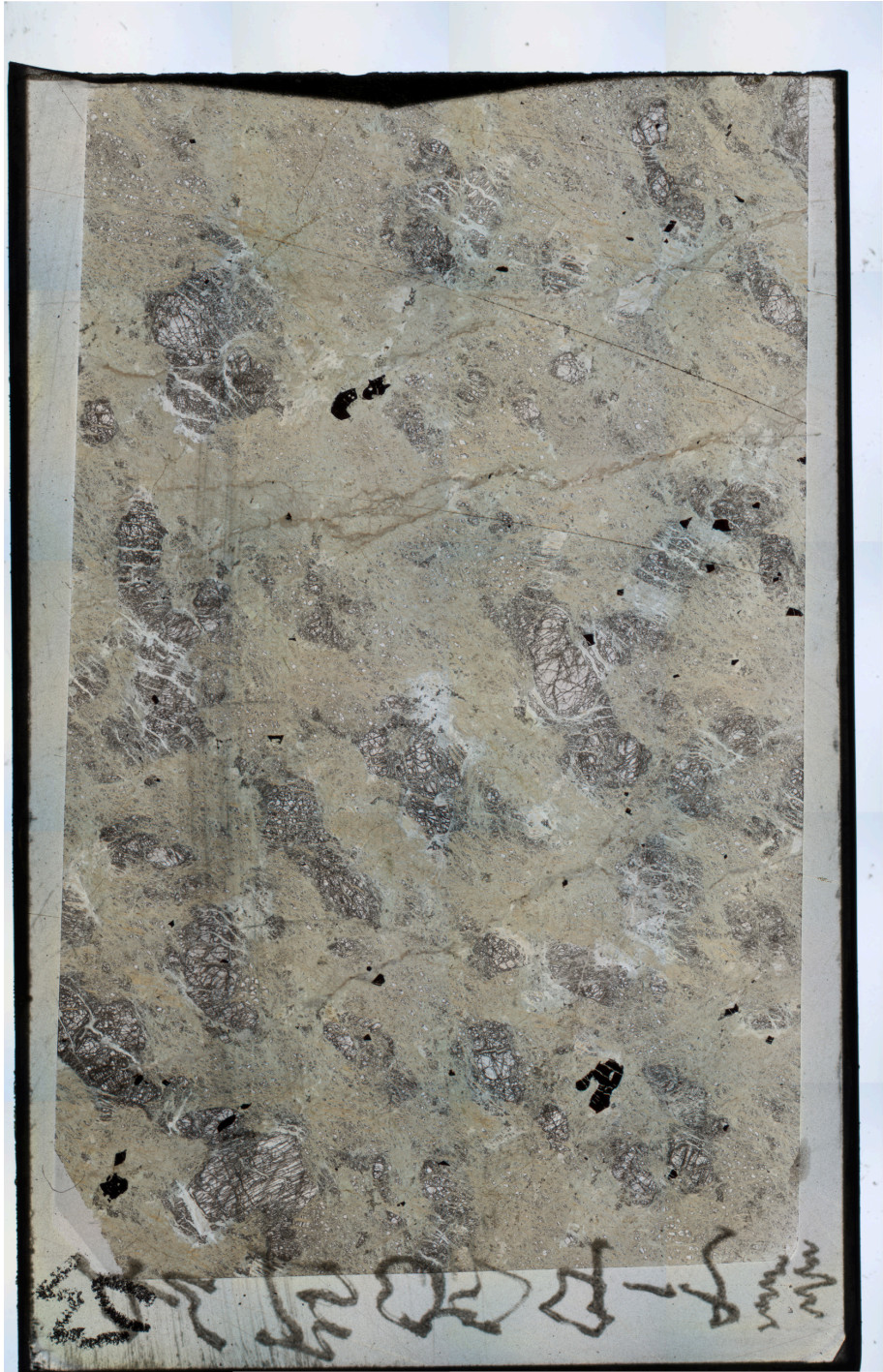
Figure A.7: Full thin section photograph of sample ALB09-1 (serpentinized harzburgite).
