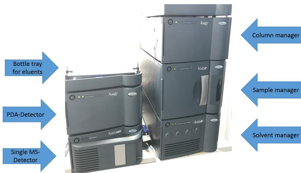
Fig. 4: Example of modular LC system in typical method development configuration
