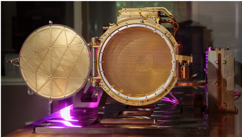
FIGURE 17. The SURface Dust Analyzer (SUDA) flight model. From Kempf et al. [215].
