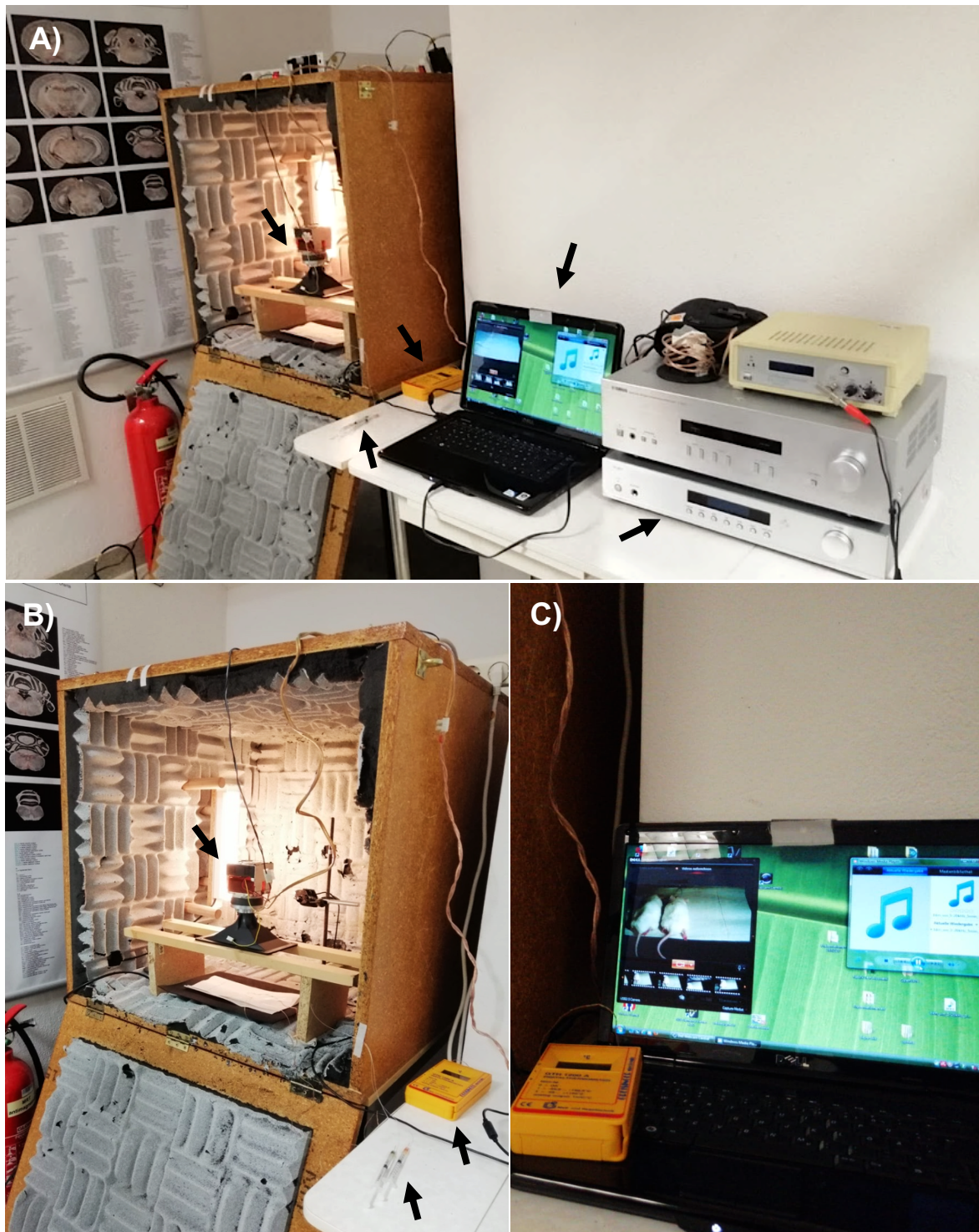
Figure 6. Noise exposure paradigm. (A-B) Noise exposure setup: animals were noise exposed to broadband white noise (5-20kHz) at different intensities (115 dB or 90 dB SPL) for 3h inside a soundproof chamber. Noise was delivered binaurally by a speaker connected to an audio amplifier and a DVD player. The speaker was placed right above the animal's head, held by wooden bars. The loud noise speaker was cooled down using a ventilator placed above the speaker. The temperature inside the chamber was constantly monitored using a temperature probe and kept between 38-36 °C. Two syringes connected to two catheters were placed outside the chamber in order to deliver 30% of the original anesthetic every 30 minutes in order to keep the anesthetized state of the animals. The catheters were correctly labelled and placed subdermally. SPL levels were adjusted with our audio amplifier and calibrated until the desired levels using a sound level meter. (C) The activity of the animals was constantly monitored using a video camera that allowed the observation of breathing respiration patterns.
