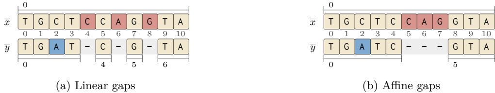
Figure 2.3: Effects of choosing either linear (a) or affine gap score functions (b). The three single deletion events in a are condensed into a single deletion event of size three in b.
