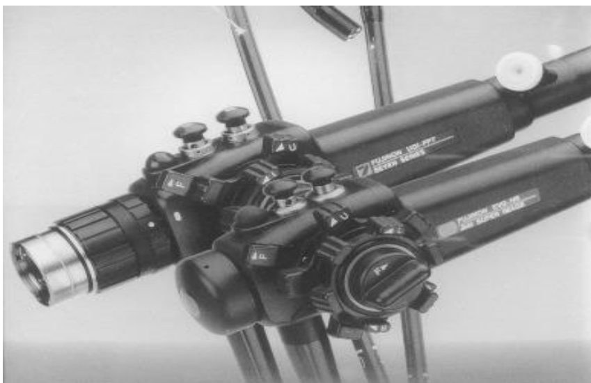
Fig. 10 Fujifilm fiberoptic panendoscope (top) and videopanendoscope (bottom), 1990. (Source: Achord, J.L. and V.R. Muthusamy, The history of gastrointestinal endoscopy, in Clinical gastrointestinal endoscopy. 2019, Elsevier. p. 2-11. e1, used with friendly permission.)
