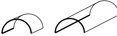
Figure 4.2: Two examples of the construction of the Minkowski sum of a line segment and a circular arc.
