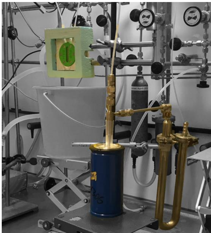
Figure 166: Setup of the in-situ XAFS cell with a mobile HF deactivation (brass-colored highlights). I recommend the flame-sealing of the HF inlet after filling of the cell and cooling the bubbler containing the perfluorinated hexanes (98 %, 85 % n -isomer, ABCR) at \vartheta = 0 °C. All parts in contact with HF were made from fluoroplastics or stainless steel. The mobile HF deactivation was used for the low temperature XAFS cell for reference measurements of \text{NiF}_4 and \text{NiF}_3 as well.
