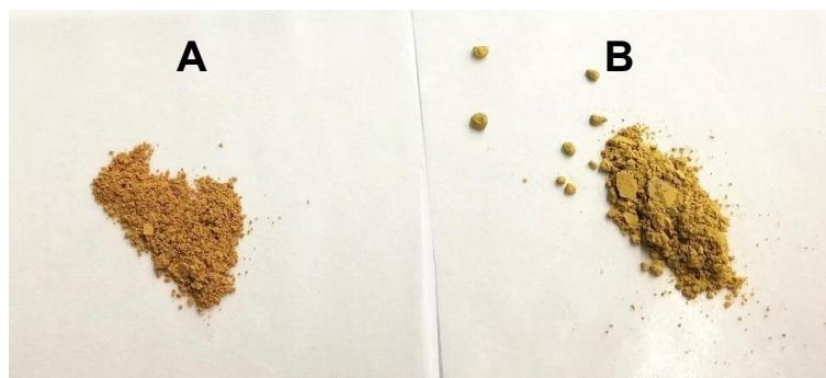
Figure S9. Fresh CN-OA-m (A) and CN-OA-m after six recycling experiments (B).
