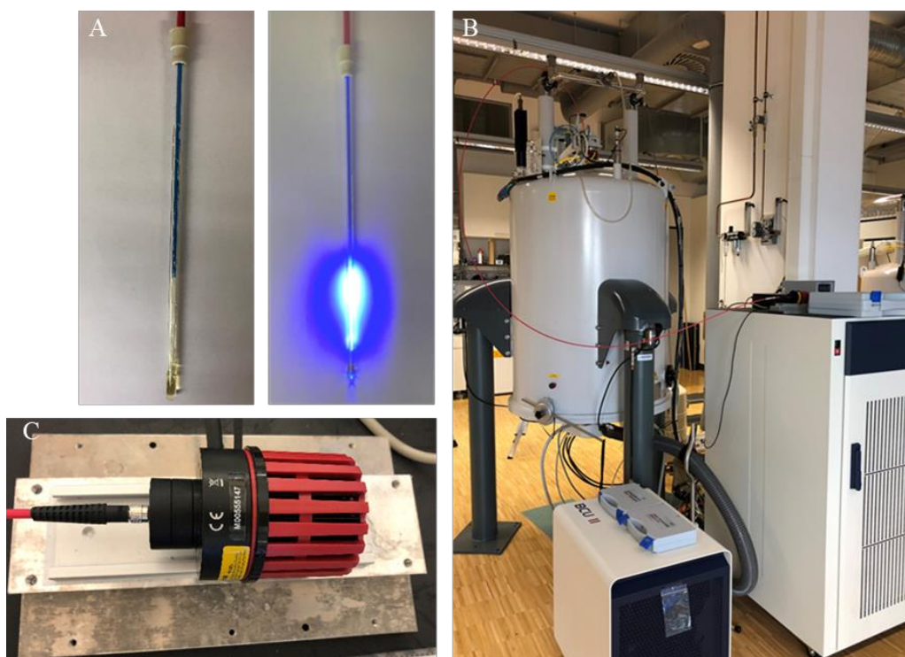
Figure S10: (A) Optic fiber inside a NMR tube (inner diameter 2.1 mm) embedded in a NMR tube (inner diameter 4.0 mm) sealed with a septum. (B) Varian 600 Spectrometer (600 MHz, Bruker). (C) THORLABS M450LP1 lamp with optic fiber attached.
