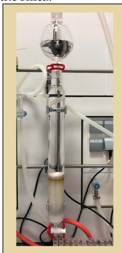
Figure 4. Glass column loaded with a slurry of silica, the crude product, and sea sand, eluted with ethyl acetate and hexane.
