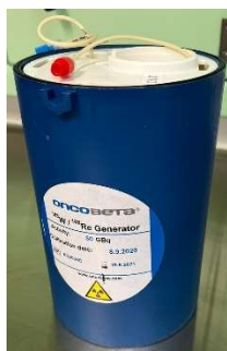
Scheme 2: ^{188}\text{W}/^{188}\text{Re} generator and production and decay scheme of ^{188}\text{Re} .
