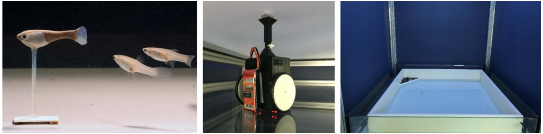
Figure 1. The RoboFish system. The 3D printed fish replica is attached to a magnetic base plate (left panel). Its movements are controlled by a two-wheeled robot below the fish tank carrying a neodymium magnet (middle panel). The tank is a quadratic ( 1\text{ m} \times 1\text{ m} ) with a triangular start box used as shelter for the live fish at the beginning of a test trial (right panel). The robot control software tracks the position and orientation of both the live fish and the robot in real-time (see section 2).
