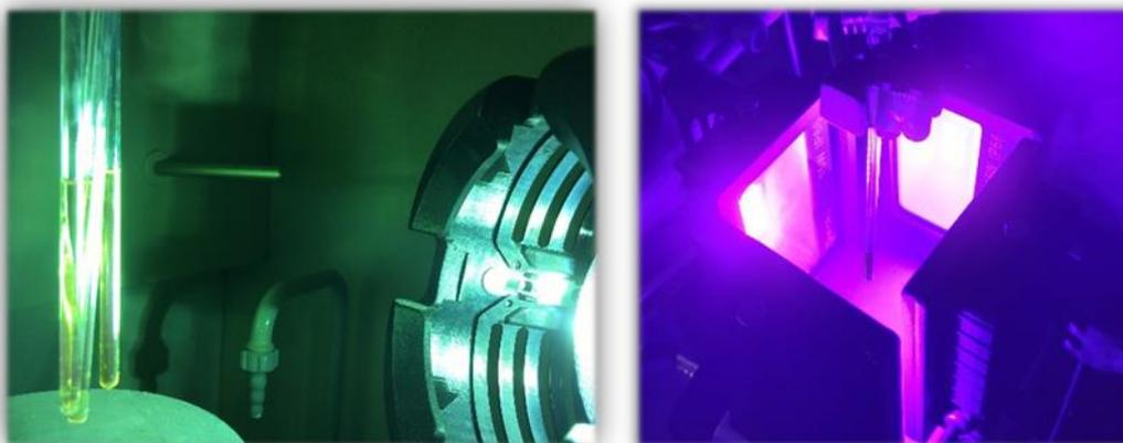
**Figure 77.** The UV mercury high-pressure lamp (100 W,  $\lambda_{\max} = 365$  nm) irradiating three NMR samples (left) and the setup of four violet light ("blacklight") LED arrays (4x 15 W,  $\lambda_{\max} = 405$  nm) irradiating one NMR samples in the middle (right).
