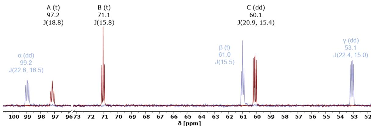
**Figure 65.**  $^{31}\text{P}\{^1\text{H}\}$  NMR spectra of [(dippe)Pd(MesCP)] (**184**, red) and [(dcpe)Pd(MesCP)] (**185**, blue) in tetrahydrofuran- $d_8$ .
