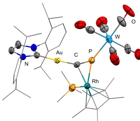
**Figure 21.** Molecular structure of **1.38** in the crystal. Anisotropic displacement ellipsoids are shown at 50% probability level. Hydrogens omitted and carbon atoms of the ligands partly reduced for clarity.
