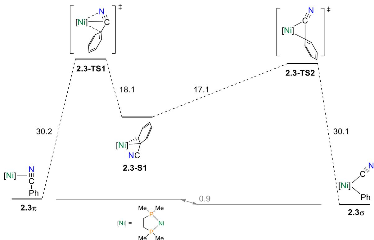
**Scheme 16.** Energetics of the C-CN bond cleavage in benzonitrile. Free energies in kcal·mol<sup>-1</sup> relative to the total energies of the fragments ([Ni(dmpe)] and PhCN).
