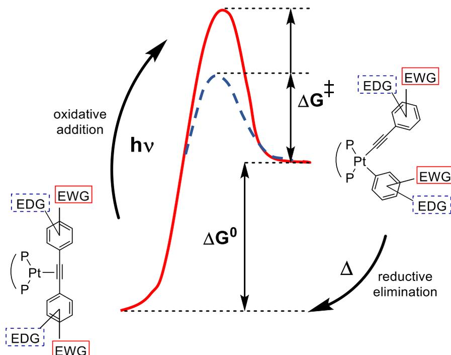
**Scheme 22.** Energetics of the photochemical oxidative  $C(sp^2)$ - $C(sp)$  bond cleavage and the thermal reductive elimination.<sup>[274]</sup>
