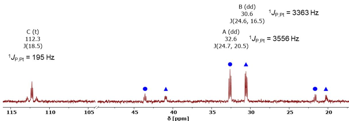
**Figure 57.**  $^{31}\text{P}\{^1\text{H}\}$  NMR spectrum of  $[(\text{dippdmea})\text{Pt}(\text{MesCP})]$  (**160**) in tetrahydrofuran- $d_8$ . The blue dots and triangles assign the  $^{195}\text{Pt}$  satellites of the dippdmea phosphorus signals.
