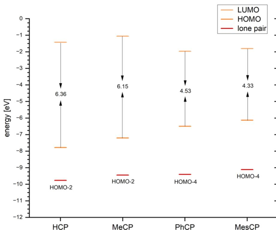
**Figure 36.** Calculated HOMO and LUMO energy levels as well as the phosphorus lone pairs for selected phosphaalkynes.
