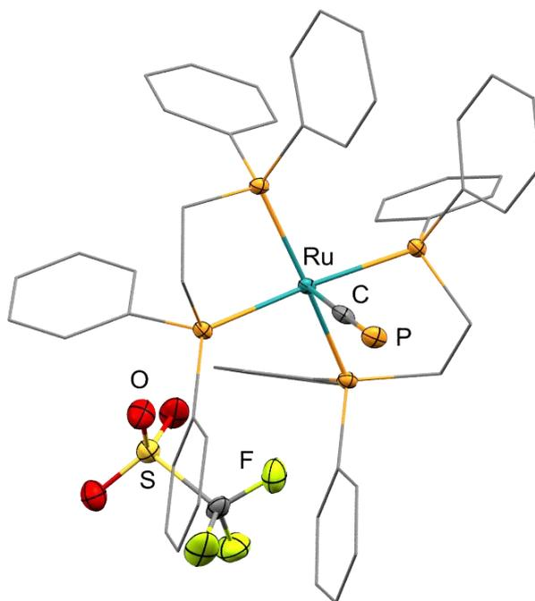
**Figure 16.** Molecular structure of **1.31** in the crystal. Anisotropic displacement ellipsoids are shown at 50% probability level. Hydrogens and co-crystallized toluene omitted. Carbon atoms of the dppe ligands reduced for clarity.
