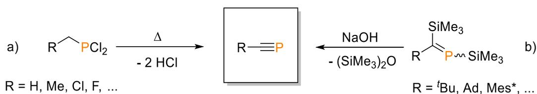
**Scheme 67.** Common synthesis of phosphalkynes by double elimination of HCl from a dichlorophosphine (a) or hexamethyldisiloxane elimination of a phosphalkene (b).
