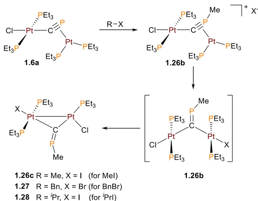
**Scheme 12.** Proposed mechanism for the methylation/alkylation of **6a**.
