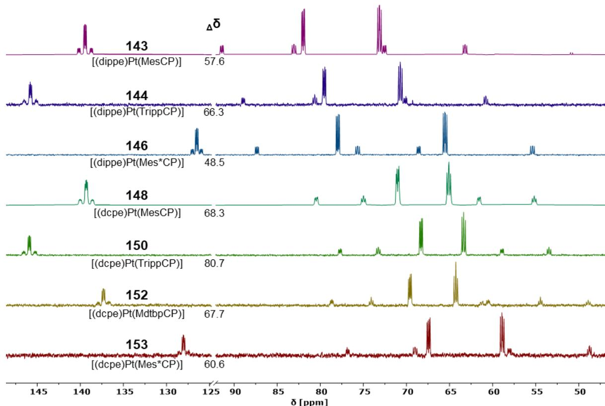
**Figure 62.**  $^{31}\text{P}\{^1\text{H}\}$  NMR spectra of the synthesized  $\text{C}_2$  arylphosphaalkyne platinum complexes. The  $\Delta\delta$  [ppm] value is the shift difference between the  $\text{C}\equiv\text{P}$  phosphorus signal and the highest shifted (left) phosphorus of the diphosphine.
