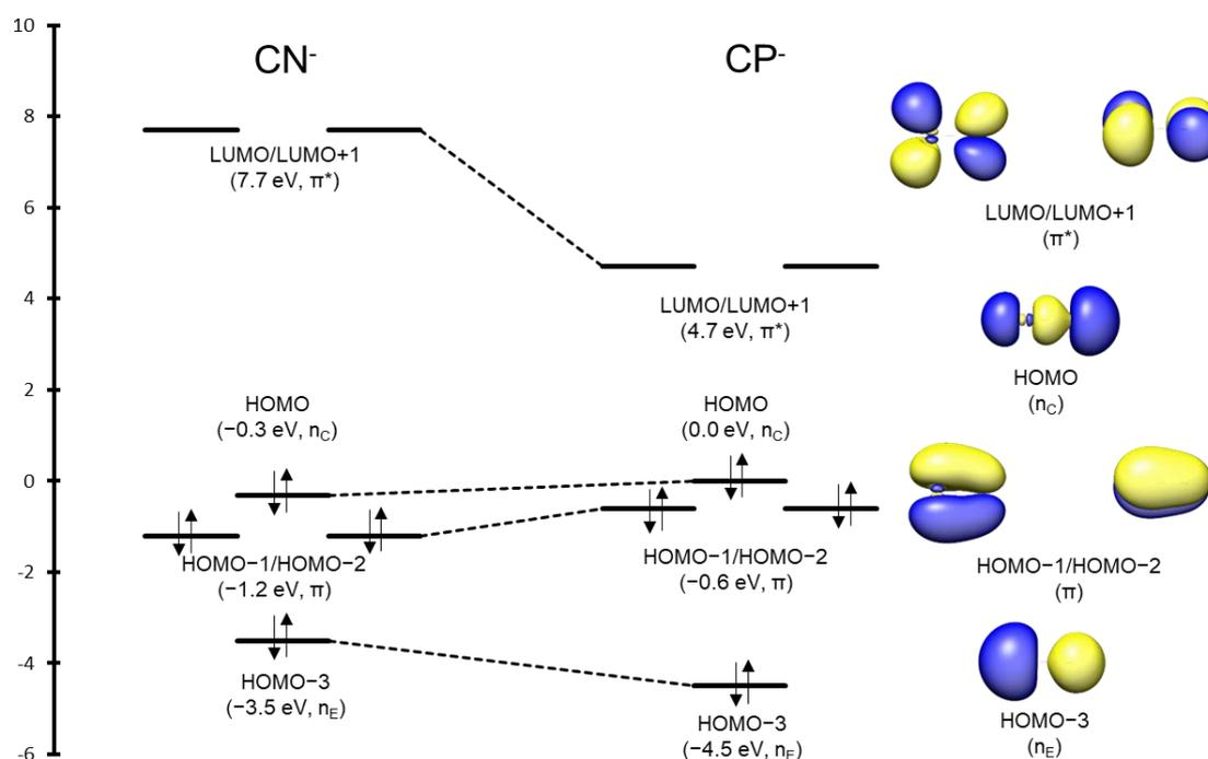
**Figure 68.** MO Scheme for  $\text{CN}^-$  and  $\text{CP}^-$  (left) and selected MOs of  $\text{CP}^-$  (right).
