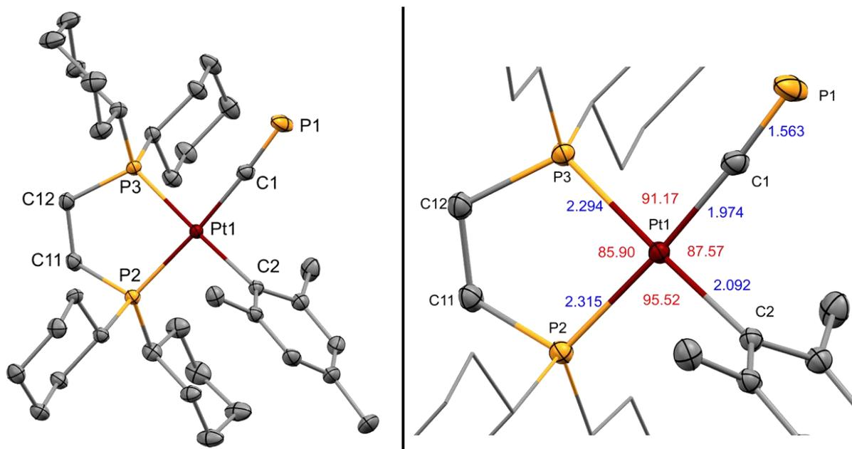
**Figure 79.** Molecular structure of [(dcpe)Pt(CP)(Mes)] (**148 $\sigma$** ) in the crystal. Anisotropic displacement ellipsoids are shown at 50% probability level. Hydrogens omitted for clarity. Selected bond lengths (Å) in blue and angles (°) in red.
