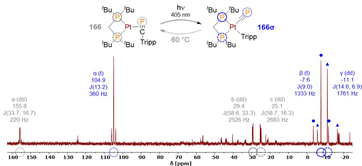
**Figure 86.** Resulting  $^{31}\text{P}\{^1\text{H}\}$  NMR spectra of a 1:3 mixture of  $[(\text{dtbpm})\text{Pt}(\text{TrippCP})]$  (**166**) and  $[(\text{dtbpm})\text{Pt}(\text{CP})(\text{Tripp})]$  (**166 $\sigma$** ) after irradiation of **166** in THF with violet light ( $\lambda_{\text{max}} = 405$  nm) for 48 h. The dtbpm  $^{195}\text{Pt}$  satellites of **166 $\sigma$**  are marked with blue dots and triangles. Circles tag the corresponding phosphorus nuclei.
