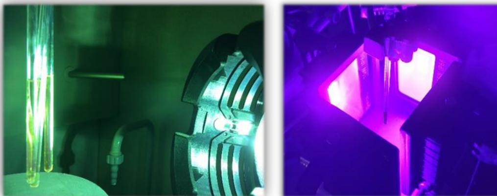
**Figure 77.** The UV mercury high-pressure lamp (100 W,  $\lambda_{\text{max}} = 365 \text{ nm}$ ) irradiating three NMR samples (left) and the setup of four violet light ("blacklight") LED arrays (4x 15 W,  $\lambda_{\text{max}} = 405 \text{ nm}$ ) irradiating one NMR samples in the middle (right).
