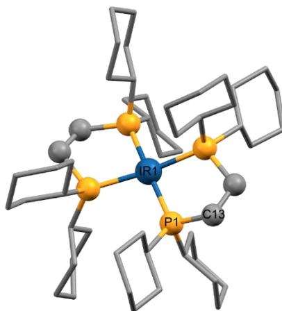
**Figure 67.** Connectivity structure of  $[\text{Ir}(\text{dcpe})_2]\text{BF}_4$  in the crystal, shown as ball-stick model. Hydrogens, four co-crystallized toluenes and  $\text{BF}_4^-$  anion omitted for clarity.
