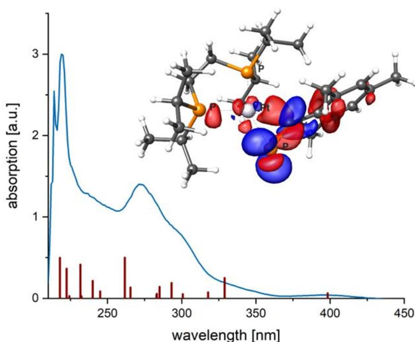
**Figure 92.** Experimental UV-Vis spectrum (blue) and theoretical vertical excitations (red) calculated with the DLPNO-STEOM-CCSD method for [(dippe)Pt(MesCP)] (**143**). Density difference plot (isosurface value 0.003) for the transition at  $\lambda = 398.3$  nm for **143** with MLCT ( $d_{x^2-y^2} \rightarrow \pi^*_{\text{CP}}$ ) and LLCT ( $\pi_{\text{Mes}} \rightarrow \pi^*_{\text{CP}}$ ) as main contribution. The transition occurs from red to blue.
