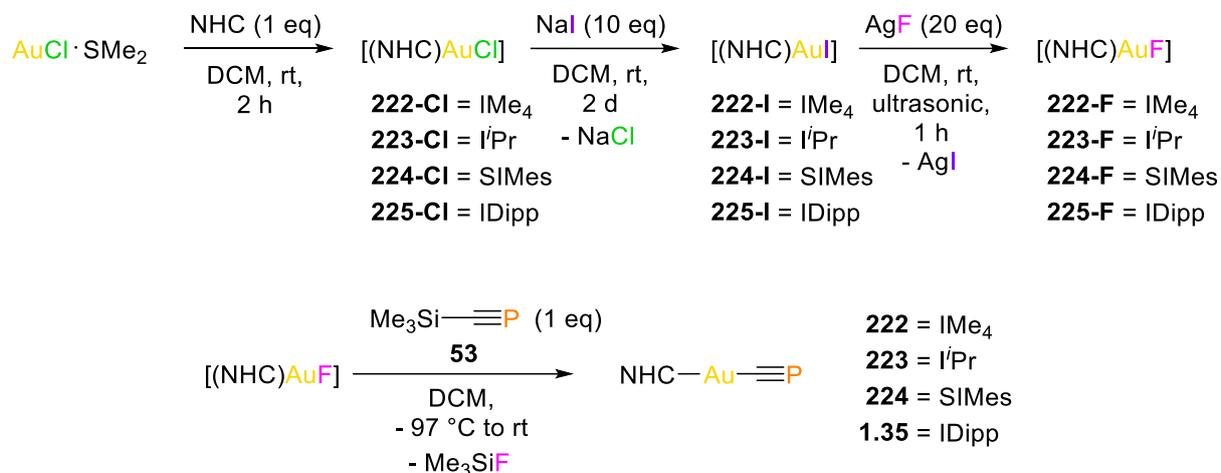
**Scheme 66.** Reaction route from  $\text{AuCl} \cdot \text{SMe}_2$  to the cyaphido gold(I) complexes **222**, **224** and **1.35**. The final reaction towards **223** was not successful.  $\text{I}^i\text{Pr}$  = 1,3-diisopropylimidazol-2-ylidene,  $\text{IMe}_4$  = 1,3-dimethylimidazol-2-ylidene,  $\text{SIMes}$  = 1,3-bis(2,4,6-trimethylphenyl)-4,5-dihydroimidazol-2-ylidene,  $\text{IDipp}$  = (1,3-bis(2,6-diisopropylphenyl)imidazol-2-ylidene).
