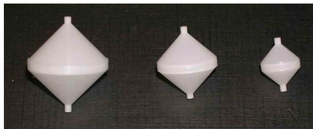
Figure 5.15: Photograph of the phantom lesions. The lesions consist of two hollow cones made of delrin. The center diameters are 20, 15, and 10 mm.
