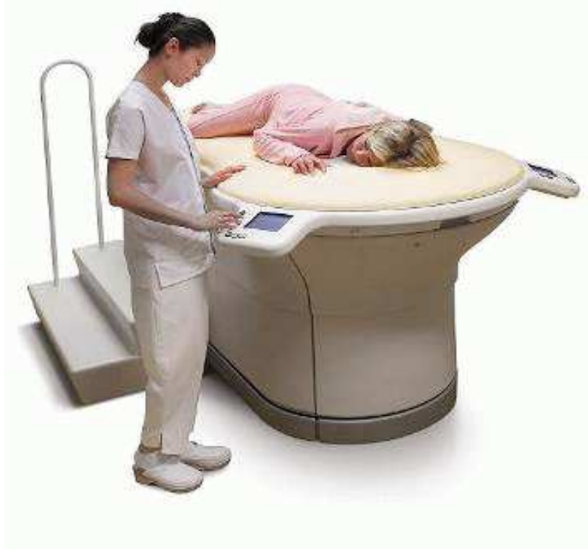
Figure A.1: Photo of Philips tomographic fluorescence mammograph. The patient is lying in prone position with one breast immersed in the fluid filled detection chamber which is mounted at the top center of the couch. The mammograph can be controlled via two identical displays attached at both front sides.
