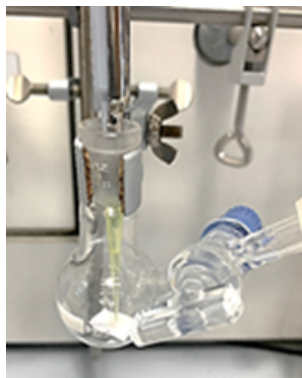
Experimental Figure 4.5: Spotting of a glycosyl donor onto a functionalized membrane, bearing a glycosyl acceptor, inside a Schlenk flask under argon counter flow.
