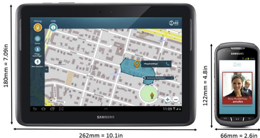
Figure 1 Tablet for care partners and smartphone for persons with dementia displaying the DCS prototype. Extracted from figure 1 found in (31).
