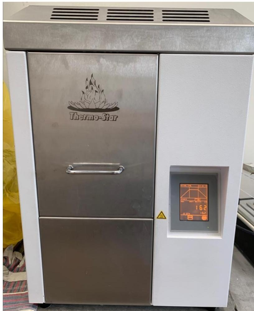
*Figure 6: The ceramic furnace (Thermo Star, Thermo-Star GmbH, Aachen, Germany) used for sintering the Zr samples.*
