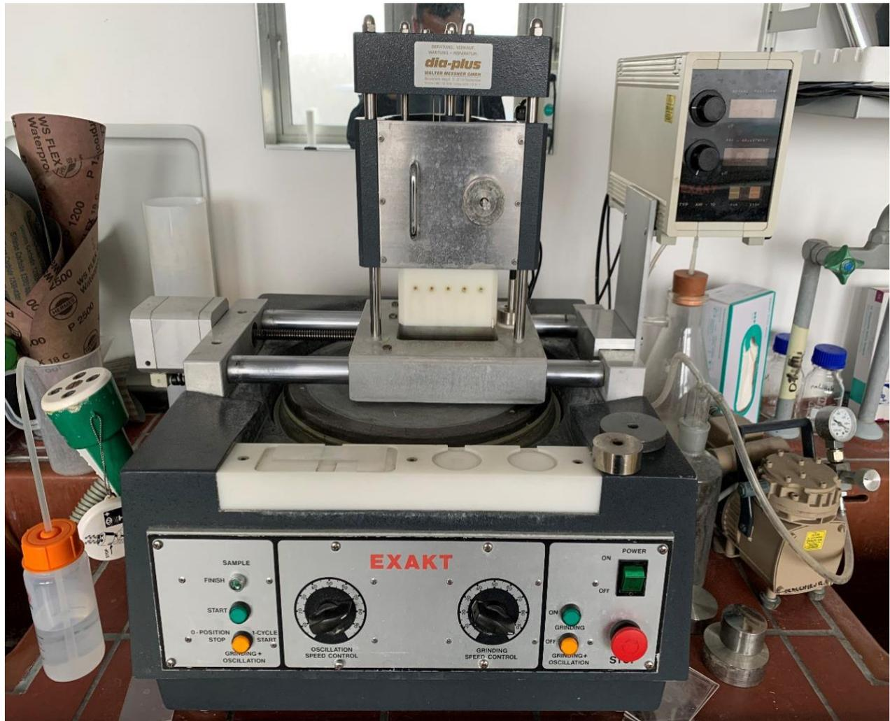
*Figure 7: The polishing machine (Exakt 400 CS, EXAKT Advanced Technologies GmbH, Norderstedt, Germany) used to polish the sample surfaces.*
