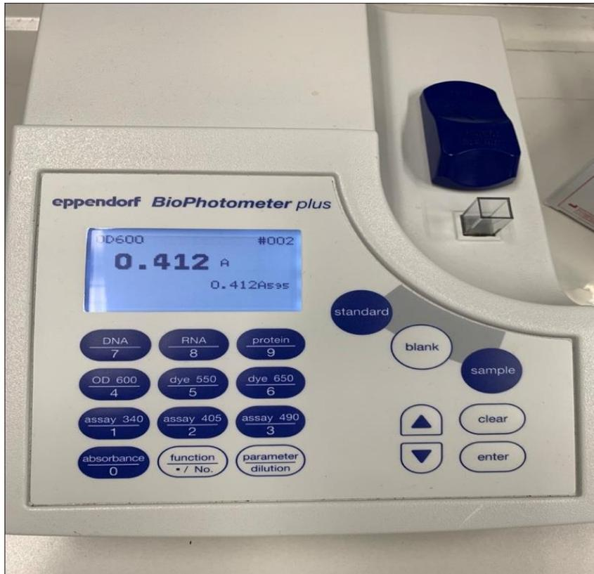
*Figure 10: The photometer (BioPhotometer Plus, Eppendorf AG, Hamburg, Germany) which was used to obtain a bacterial concentration in the TSB medium.*
