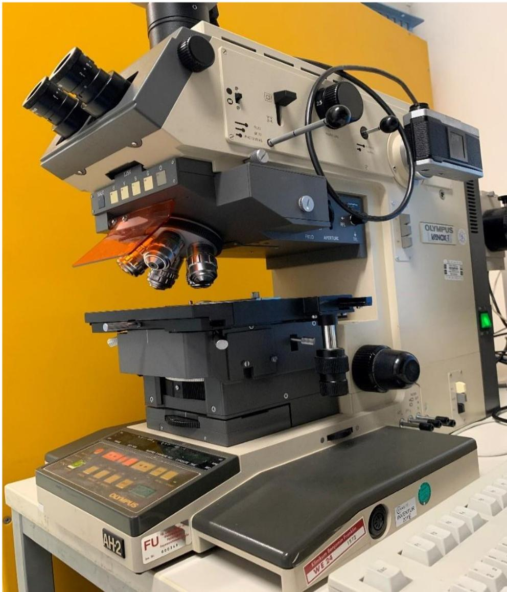
*Figure 13 : The fluorescence microscope (Vanox T AH-2 DIC, OLYMPUS EUROPA SE & CO. KG, Hamburg, Germany), which was used to visualize the *S. sanguinis* colonies after 18 hours of incubation.*
